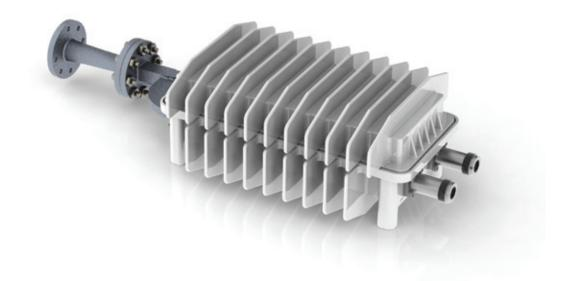
The SAGE SatCom Ka Band Transceiver provides 5 W of linear power in the most compact package available in the industry. The integration of the SAGE SatCom 5W Ka Band BUC and Ka Band LNB results in a compact and light weight assembly that allows direct mounting to the antenna feed arm. Simplifying system planning and logistics, a single model covers the complete frequency band from 29 GHz to 30 GHz. The transceiver includes built-in M&C for remote and local monitoring and control via the IF.
